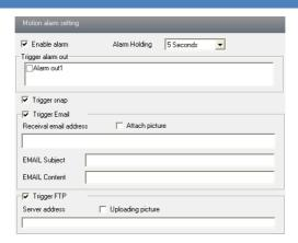
**Alarm Out**: If selected, this would trigger the external relay output on detecting a motion based alarm.
